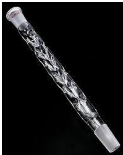
Figure 04: Vigreux column. Adapted from Labasics Colonne de Distillation Vigreux, 24/40 200 mm, by Labasics, (n.d.), Amazon.fr.
