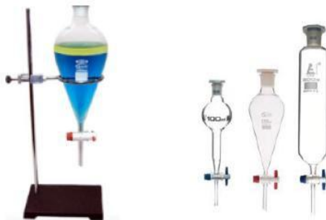
Figure 01: Different shapes of separatory funnels. Adapted from Separatory Funnel, by Home Science Tools, (2017).
