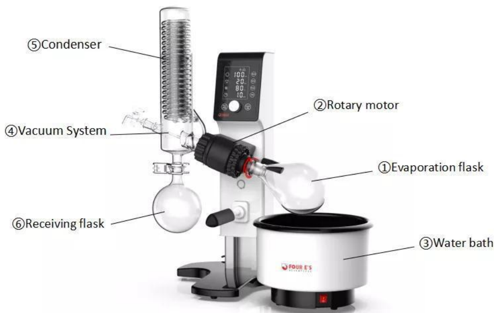
Figure 03: Main parts of a rotary evaporator. Adapted from Everything You Want to Know About Rotary Evaporator, by FOUR E's Scientific, (2023).
