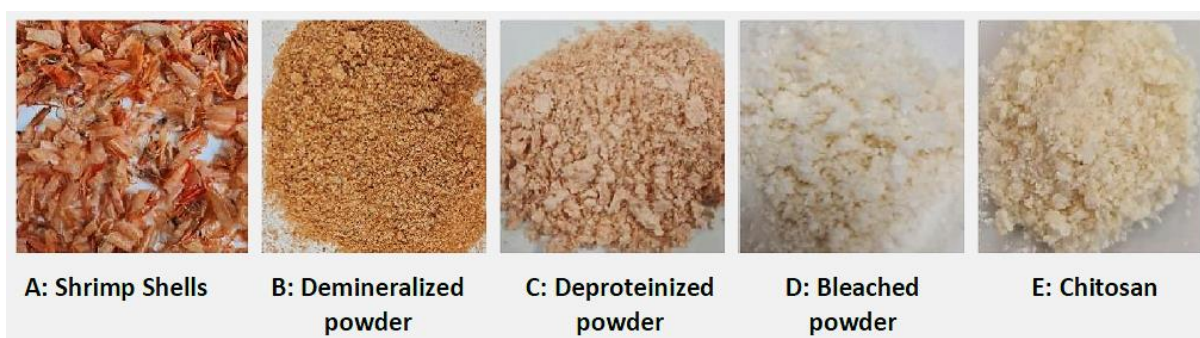
Figure 06 : Comparison of Colloidal Chitin, Demineralized Chitin, Deproteinized Chitin, and Chitosan from Shrimp Shells
