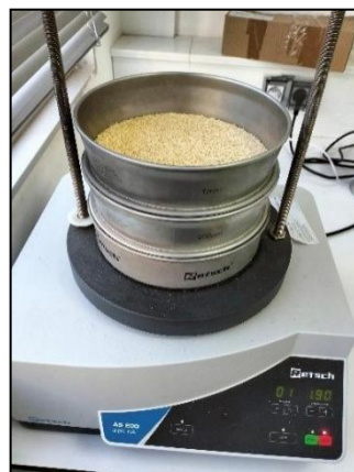
Figure 4: Sieving dried sawdust
